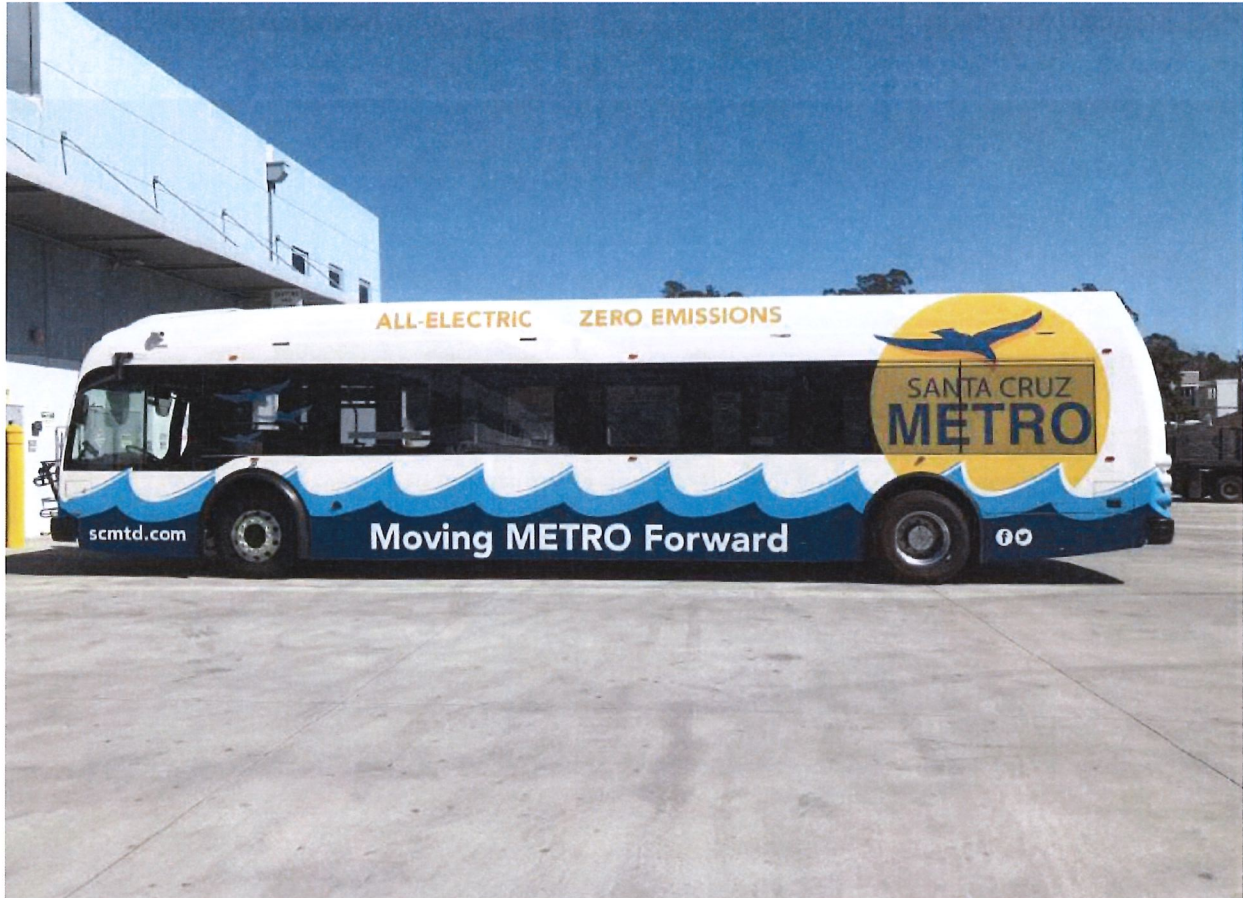
Equipped with 660kwh of energy storage, the 40-foot Proterra ZX5 can deliver up to 329 miles of drive range. Photo courtesy Santa Cruz Metro
